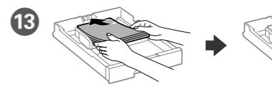
Load A4 size paper toward the back of the paper cassette with the printable side face down then slide the front edge guide to the paper.
