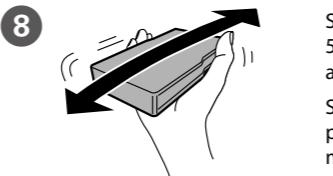
Shake the ink cartridge horizontally for 5 seconds, moving it back and forth about 10 cm 15 times.
